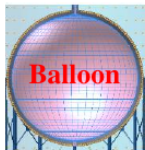
Nylon (ETFE) balloon in LAB in a stainless steel sphere
