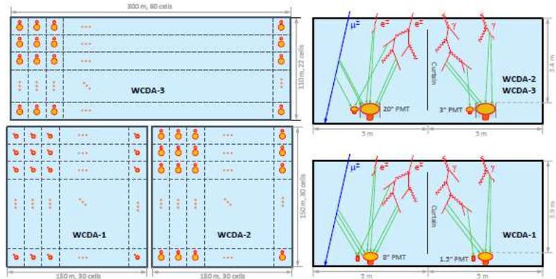
Figure 6: Layout sketch of the LHAASO-WCDA (left) and side views of two cells (right). In the left panel, two sets of circles in each cell partitioned by black dashed lines denote the big and the small PMTs, and the black dashed lines represent the plastic curtains. The water depth over the PMT top surface is 3.9 m and 3.4 m for WCDA-1 and WCDA-2 & 3, respectively.
